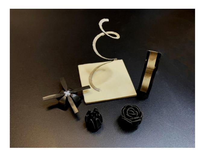
An assortment of objects made from magnetic shape-memory polymers. Credit: Shuai Wu, The Ohio State University
