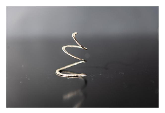
This object is made from a special material called "magnetic shape-memory polymer." It can bend and change shape in response to a magnetic field. Credit: Allison Carter
