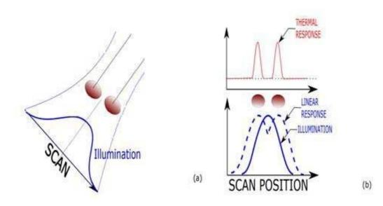
Scanning illumination, thermal response and super-resolution factor. (a) Two objects are illuminated by a scanning focused energy source with a size larger than the objects or the distance between them. (b) The thermal light emission produced by the scanning illumination and the heating of the objects is spatially compressed compared to a linear response to the illumination. Credit: Institute for Basic Science
