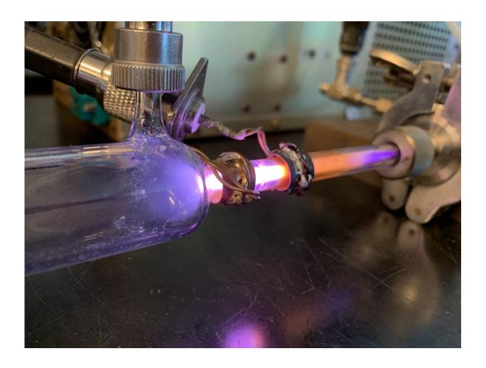
Silicon nanocrystals are formed by a silane gas in a plasma process. Credit: Lorenzo Mangolini/UC Riverside
