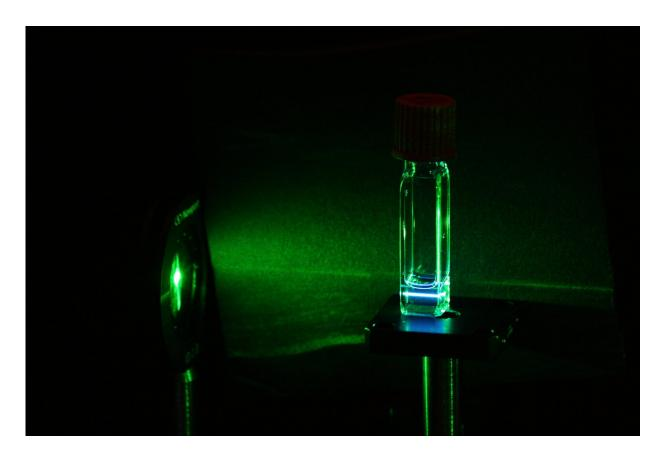
A green lower-energy laser light goes through the silicon quantum dots, which the silicon quantum dots re-emit, or upconvert, into a higher-energy blue light. Credit: Lorenzo Mangolini & Ming Lee Tang/UCR
