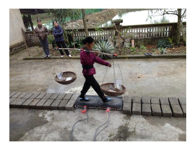
A woman carrying a heavy load on a flexible bamboo pole walking on a force plate. Credit: Bertram Lab, University of Calgary
