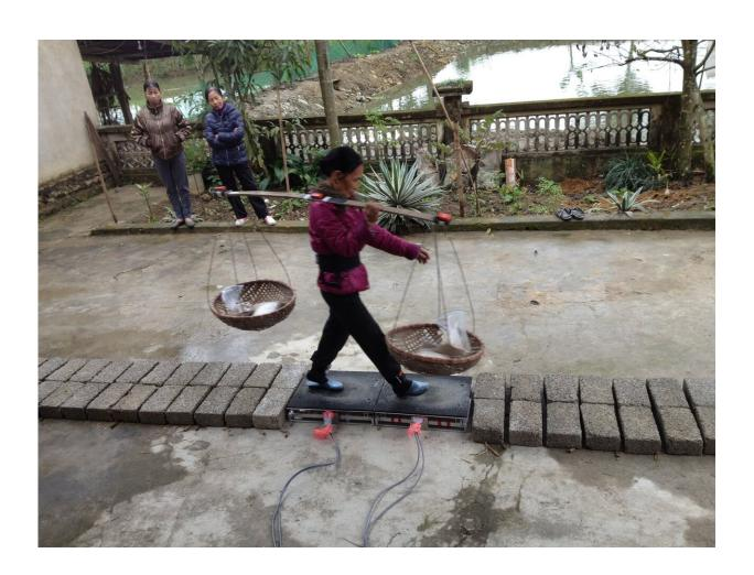
A woman carrying a heavy load on a flexible bamboo pole walking on a force plate. Credit: Bertram Lab, University of Calgary
