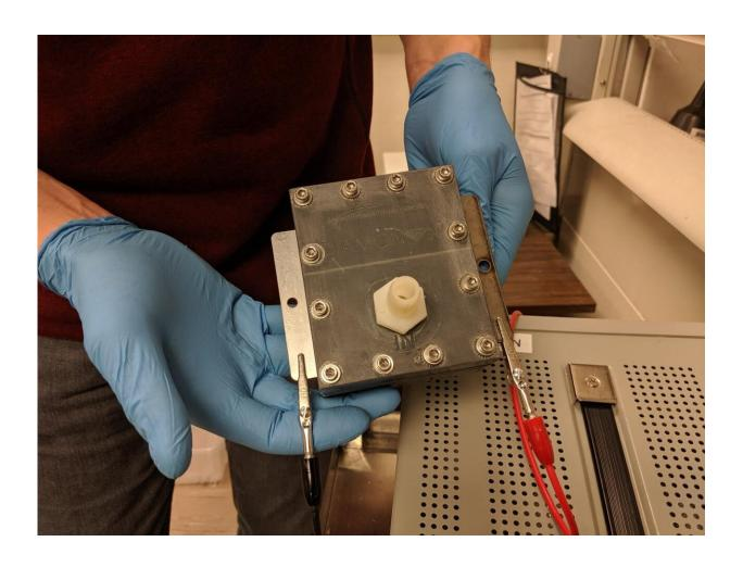
An electrochemical flow cell with a stainless steel cathode and a boron-doped diamond anode is used to treat a concentrated waste stream of GenX. Credit: Colorado State University
