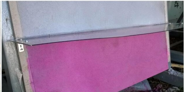
Time zero: Photocatalytic panel exposed outdoors. The purple section is treated with a pollutant (Rhodamine B). A small plexiglass roof protects the treatment from being washed away by the rain.
