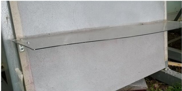
3 weeks later: The purple colour has disappeared. The pollutant has been degraded by the action of the photocatalyst under solar light.
