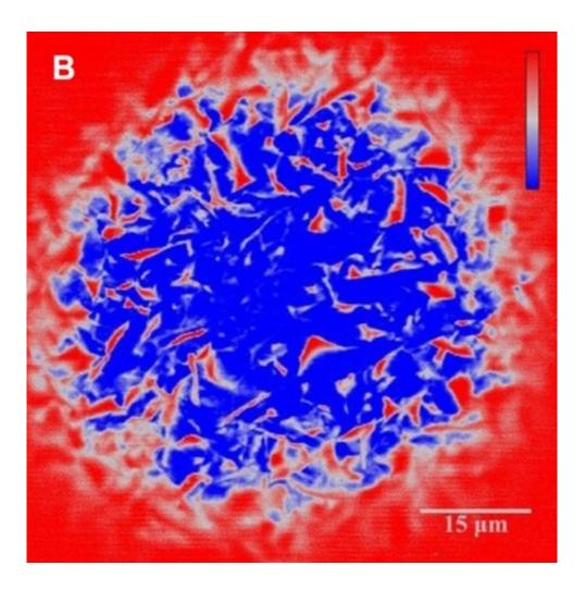
Fluorescence intensity image of the contact between a polystyrene sphere and the glass substrate. The scale bar indicates fluorescence intensity gradient from the lowest (blue) to the highest (red) values. Blue regions correspond to the load-bearing area. Credit: HIMS / Science Advances
