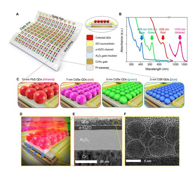
Schematic of the device structure of the QD/AOS hybrid phototransistor. (A) A schematic three-dimensional view of a phototransistor array. (B) Optical absorption of QDs used to fabricate the full-color detectors. (C) PbS QDs (10
