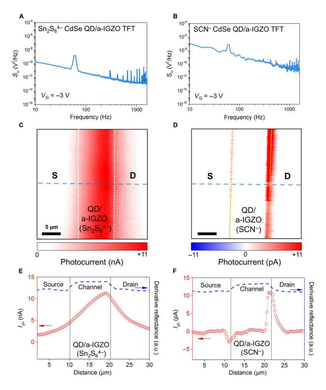
Interfacial properties between QDs and the AOS channel layer. (A and B) Noise power spectral density of 7-nm CdSe QD/a-IGZO with SCN- and Sn2S64-ligand phototransistors. (C and D) Scanning photocurrent imaging (0 V source per drain bias) of the QD/a-IGZO phototransistor with Sn2S64- and SCN-
