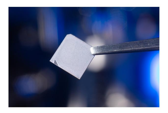
A barium zirconium sulfide thin film created by the research team. Credit: Douglas Levere / University at Buffalo
