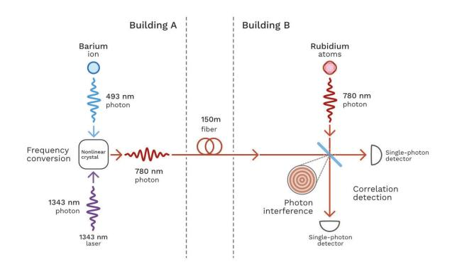
A schematic of an interference experiment in which two photons are produced in different buildings, are generated by different sources and have different colors. Credit: S. Kelley/NIST
