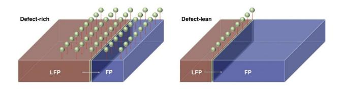
An illustration shows a battery's cathode undergoing phase transition from iron phosphate (FP) to lithium iron phosphate (LFP) during charging. Simulations by Rice University scientists showed that adding defects -- distortions in their crystal lattices -- could help batteries charge faster. Credit: Kaiqi Yang/Rice University
