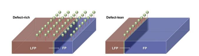
An illustration shows a battery's cathode undergoing phase transition from iron phosphate (FP) to lithium iron phosphate (LFP) during charging. Simulations by Rice University scientists showed that adding defects -- distortions in their crystal lattices -- could help batteries charge faster. Credit: Kaiqi Yang/Rice University
