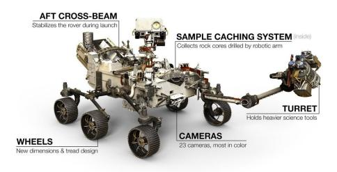
NASA's Mars 2020 rover looks virtually the same as Curiosity, but there are a number of differences. One giveaway to which rover you're looking at is 2020's aft cross-beam, which looks a bit like a shopping cart handle. JPL is building and will manage operations of the Mars 2020 rover for the NASA Science Mission Directorate at the agency's headquarters in Washington. Credit: NASA/JPL-Caltech
