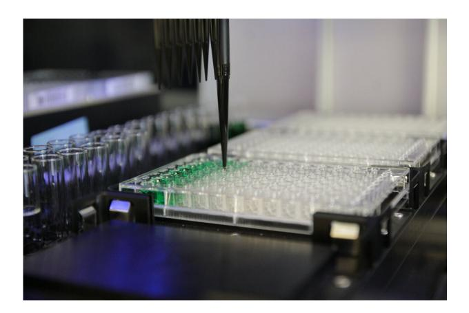
A Rutgers-led team adapted advanced liquid handling robotics to perform the chemistry required for synthesizing synthetic polymers. This new automated approach enables the rapid exploration of new materials valuable in industry and medicine. Credit: Matthew Tamasi
