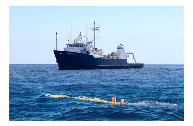
This study used two echosounders—one mounted on the research vessel New Horizon and the other on a Remus-class underwater vehicle. Credit: John Calambokidis
