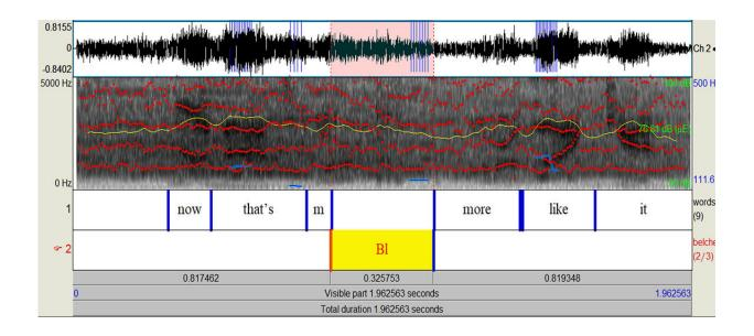
Depiction of a belched word on a waveform and spectrogram using the phonetics software Praat . Credit: Brooke Kidner
