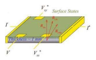
Transport measurement geometry: measuring a freshly cleaved V:BSSTS surface. Credit: FLEET
