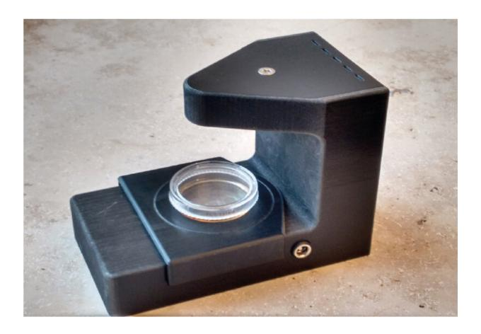
The holographic microscope enables automatic, three-dimensional tracking of immune cells in real time. Credit: Fraunhofer-Gesellschaft
