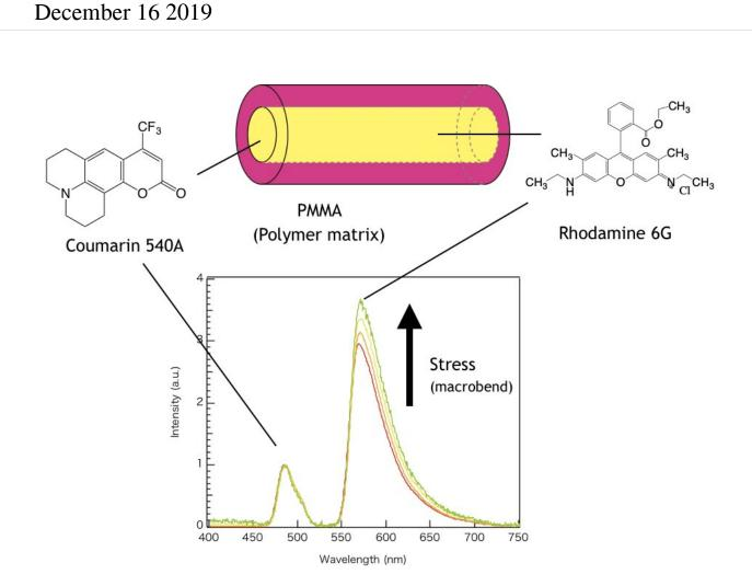
Transition of output spectrum of a fluorophore-doped polymer optical fiber upon applied stress. Credit: University of Electro Communications
