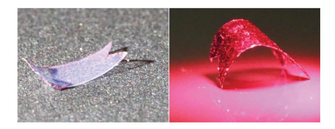
Light makes the conditioned liquid crystal move. Credit: Aalto University, Tampere University, Cell Press
