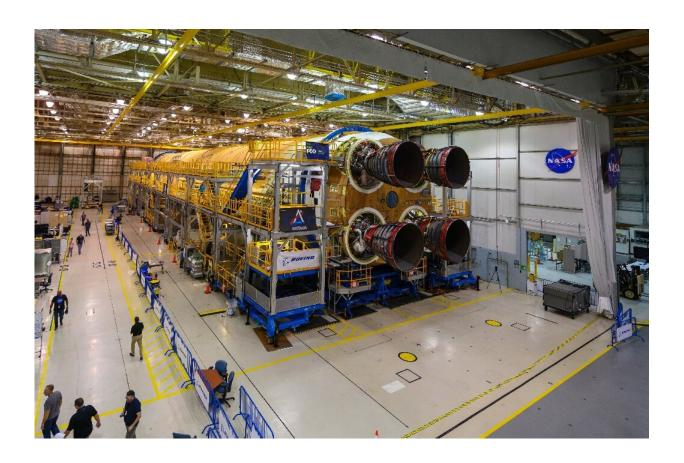
This NASA image obtained December 9, 2019 shows engineers and technicians as they attach the last of four RS-25 engines that will provide the necessary thrust for the SLS rocket to reach space, to complete assembly of the stage
