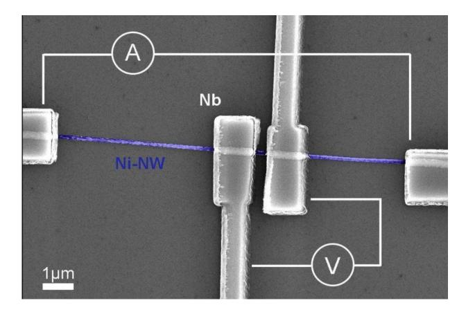
The structure microphoto. Grey at the center: superconducting niobium electrodes; blue: a ferromagnetic nickel nanowire. Graduation: 1  $\mu m$ . A and V (ammeter and voltmeter) indicate the type of current passing through the sample. Credit: O. V. Skryabina et al., Scientific Reports
