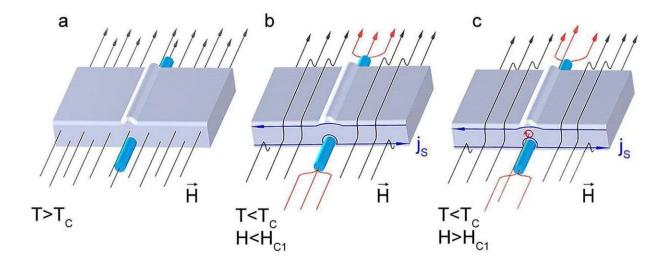
The processes occurring in the niobium (grey block) / nickel nanowire (blue cylinder) system under various ambient conditions. (a) The temperature is above critical. The system is in its normal state, the magnetic field (black arrow) is passing through the entire sample. (b) The temperature is below critical. When Hc Hc1 is exceeded, an Abrikosov vortex penetrates the niobium (marked with the red circle.) . Credit: O. V. Skryabina et al., Scientific Reports
