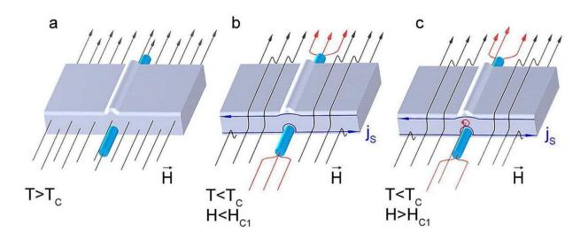
The processes occurring in the niobium (grey block) / nickel nanowire (blue cylinder) system under various ambient conditions. (a) The temperature is above critical. The system is in its normal state, the magnetic field (black arrow) is passing through the entire sample. (b) The temperature is below critical. When Hc Hc1 is exceeded, an Abrikosov vortex penetrates the niobium (marked with the red circle.). Credit: O. V. Skryabina et al., Scientific Reports
