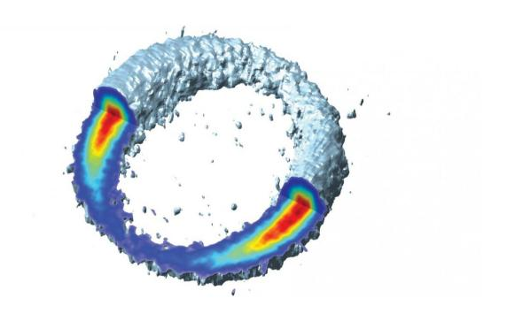
Reconstructed 3D photoelectron momentum distribution, together with a sketch of the polarisation ellipse and the beam direction. (Adapted from Willenberg et al., Nat. Commun. 10, 5548; 2019) Credit: ETH Zurich, D-PHYS, Keller group
