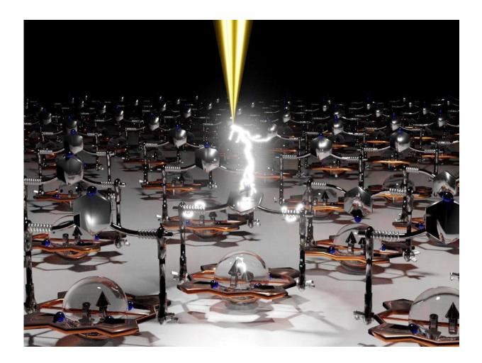
Each molecule can be separately addressed with a scanning tunneling microscope and switched between the states by applying a positive or negative voltage. Credit: Jan-Simon von Glasenapp and Rainer Herges
