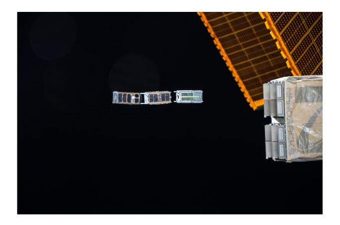
The NanoRacks CubeSat Deployer attached to the outside of the Japanese Kibo laboratory module is shown as it ejects three CubeSats. NASA's CubeSat Launch Initiative offers universities, high schools and non-profit organizations the opportunity to fly small satellites. Credit: NASA
