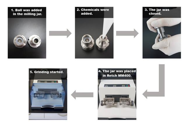
In ball milling, the chemicals and a steel ball are placed into steel jars which are then shaken vigorously. Credit: Hokkaido University
