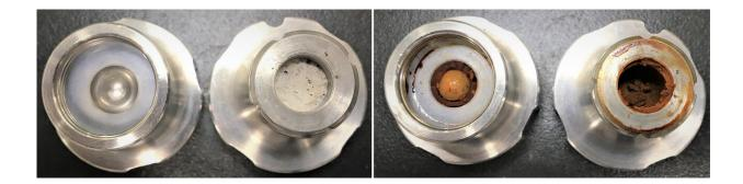
Reaction mixtures before and after grinding in a ball mill. Mechanoredox arylation reactions occurred with aryl diazonium salts and furan in the presence of a piezoelectric material (BaTiO3). (Kubota K. et al. Science, Dec. 19, 2019) Credit: Kubota K. et al. *Science*, December 19, 2019
