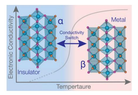
Researchers found the metal-insulator transition in the material molybdenum oxynitride occurred near 600 degrees Celsius, revealing its potential for applications in high-temperature sensors and power electronics. Credit: Northwestern University
