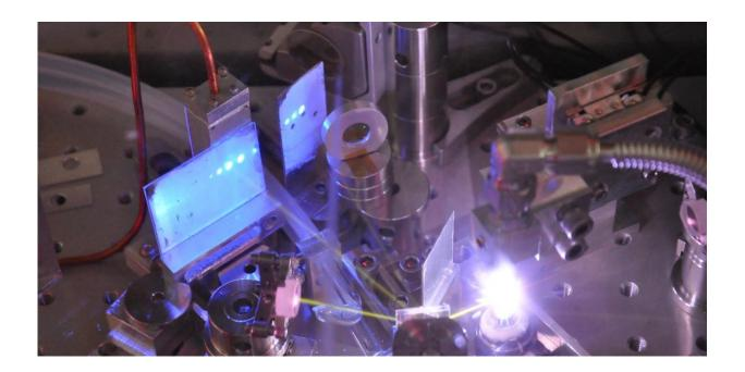
Ultrafast pulses of extreme ultraviolet light are created in a gas jet of white plasma, and are visible as blue dots on a phosphor screen as well as yellow beams from oxygen fluorescence. Credit: Research to Reality
