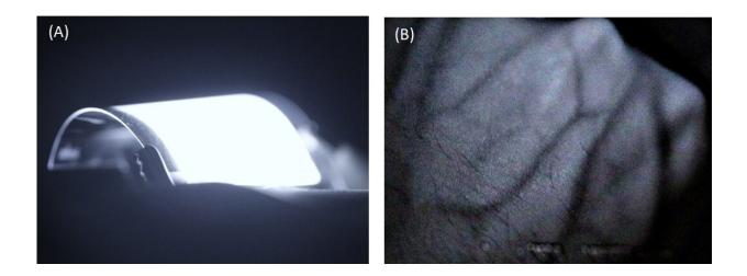
Figure (A) shows uniform electroluminescence from a large-area flexible perovskite light-emitting diode developed by the research team. Figure (B) shows illumination with near-infrared perovskite light-emitting diode on the back of the fist. This allows for the imaging of subcutaneous blood vessels. Credit: Nature Photonics
