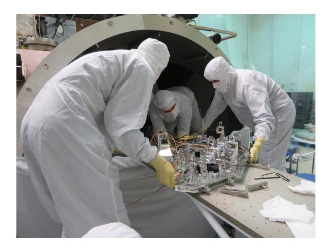
Researchers install a new quantum squeezing device into one of LIGO's gravitational wave detectors. Credit: Lisa Barsotti
