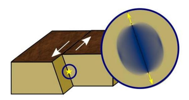
Between two solids in frictional contact, slip nucleates at a point on the surface (corresponding to the hypocenter of an earthquake) before spreading to the rest of the interface – just like a crack growing through a brittle material. Using numerical simulation, researchers computed the shear stress profile after the onset of slip and studied the drop of frictional stress observed behind the rupture fronts (blue area in the inset). Credit: Ecole Polytechnique Federale de Lausanne
