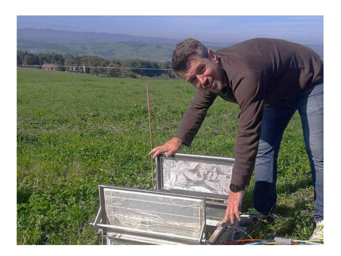
Empa researcher Erkan Ibraim controls one of the flux chambers that collect nitrous oxide emissions from the ground. Picture: Empa
