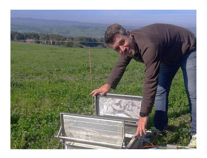
Empa researcher Erkan Ibraim controls one of the flux chambers that collect nitrous oxide emissions from the ground. Picture: Empa
