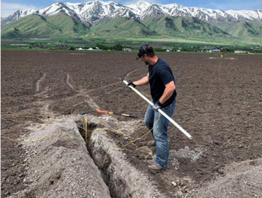
Soil moisture sensors aid in advanced irrigation scheduling and help measure water consumption on farm fields. Credit: Matt Yost
