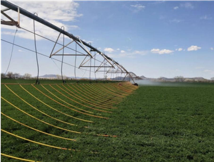
Advanced pivot irrigation systems such as mobile drip irrigation, low-energy precision application and low-energy spray application reduce wind drift and evaporation—allowing for reduced irrigation rates. Credit: Jonathan Holt
