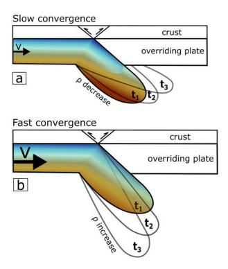
A schematic summary of the effect of the convergence rate. Upper image shows a slow convergence rate allows thermal difussion and a derived reduction of slab's density (positive buoyancy). Lower image shows how a faster convergence rate increases the slab's density promoting the negative buoyancy. Credit: Kittiphon Boonma, *Scientific Reports*
