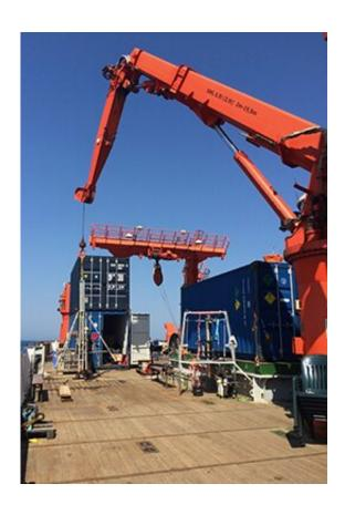
A crane is used to deploy the rig used to recover sediment cores from the seabottom. Source: W. Orsi
