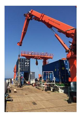
A crane is used to deploy the rig used to recover sediment cores from the seabottom. Source: W. Orsi
