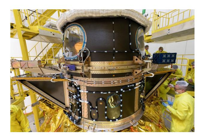
In this photo released on Saturday, Dec. 11, 2019 by the European Space Agency (ESA), the Cheops satellite, installed on the flight adapter ring is being placed on the Soyuz Fregat launch vehicle. European space officials on Tuesday, Dec. 17, 2019 postponed the launch of a three-year mission to study planets in other solar systems shortly before it was due to blast off. (M. Pedoussaut/ESA via AP)
