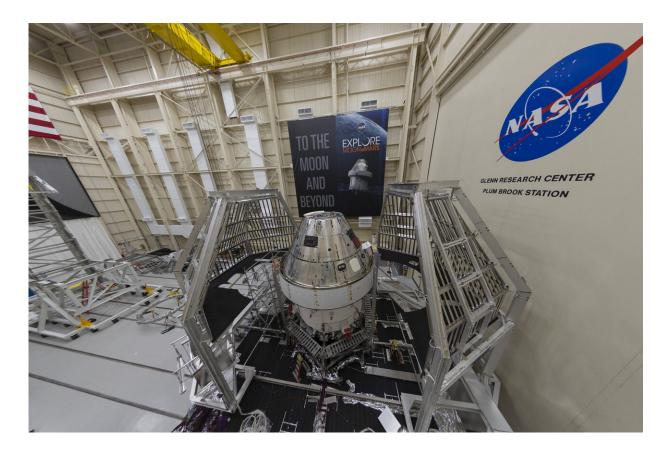
The Orion spacecraft with European Service Module at NASA's Plum Brook Station. The first Orion will fly farther from Earth on the Artemis I mission than any human-rated vehicle has ever flown before – but first it will undergo testing to ensure the spacecraft withstands the extremes of spaceflight. Credit: ESA–S. Corvaja
