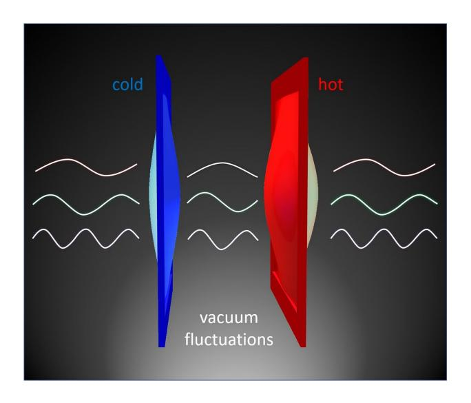
In a new study, University of California, Berkeley, researchers show that heat energy can travel through a complete vacuum thanks to invisible quantum fluctuations. In the experiment, the team placed two gold-coated silicon nitride membranes a few hundred nanometers apart inside a vacuum chamber. When
