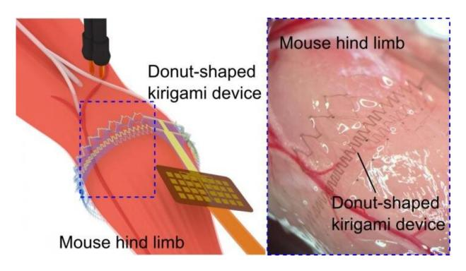
Schematic image showing the EMG signal recording (left) and photograph showing the donut-shaped kirigami device attached on the muscle surface (right). Credit: Toyohashi University Of Technology.
