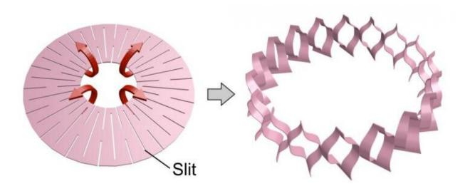
2D donut shape (left: before deformation) and 3D cylindrical shape (right: after deformation). Credit: Toyohashi University Of Technology.
