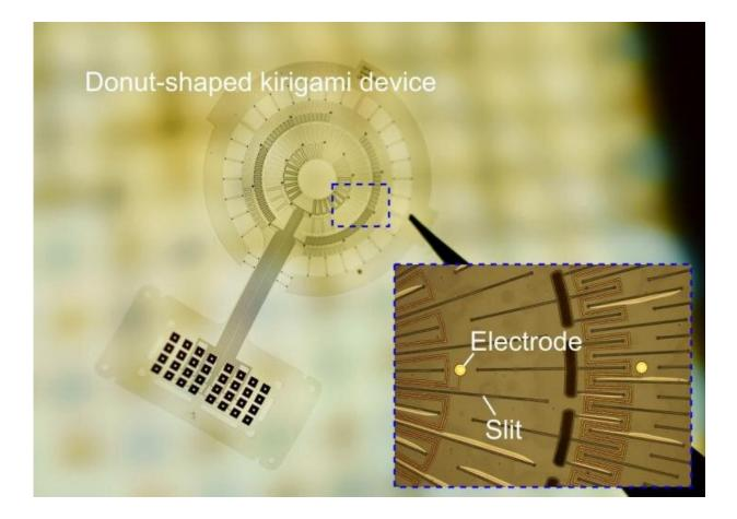
Fabricated donut-shaped kirigami device (inset: embedded electrodes). Credit: Toyohashi University Of Technology.
