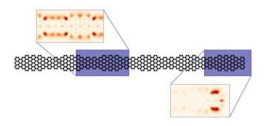
The graphene nanoribbon (center) consists of a single layer of honeycomb carbon atoms. The ribbon is only a few carbon atoms wide and has different electrical properties depending on its shape and width. The local density of the electrons is increased at the edges, as the dark red areas in the boxes show. Credit: Kiel University
