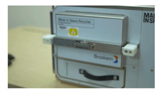
The Made in Space Recycler hardware prepared for launch to the space station to test reprocessing plastic into 3D printing filament. Credit: Made In Space, Inc.
