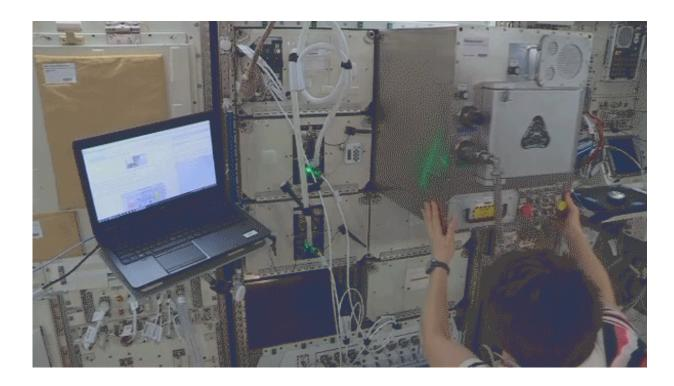
NASA astronaut Anne McClain installs the ReFabricator on the space station in Feb. 2019. The printer was developed to test technology for recycling waste plastic materials into high quality 3D-printer filament. Credit: NASA
