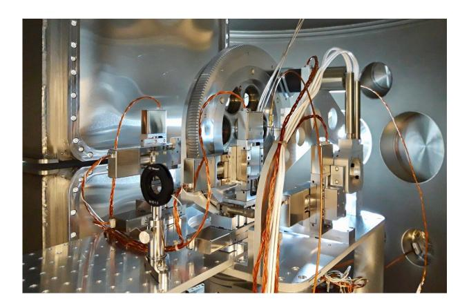
View into the interaction chamber with the revolver for up to six diamond anvil cells in the centre. Credit: DESY, Cornelius Strohm
