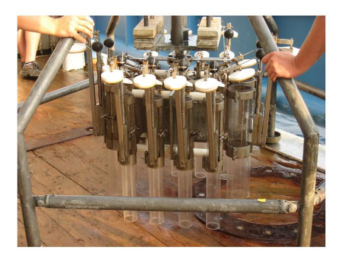
A multicorer used to take sediment samples from the seafloor. Credit: Sabine Lengger, University of Plymouth
