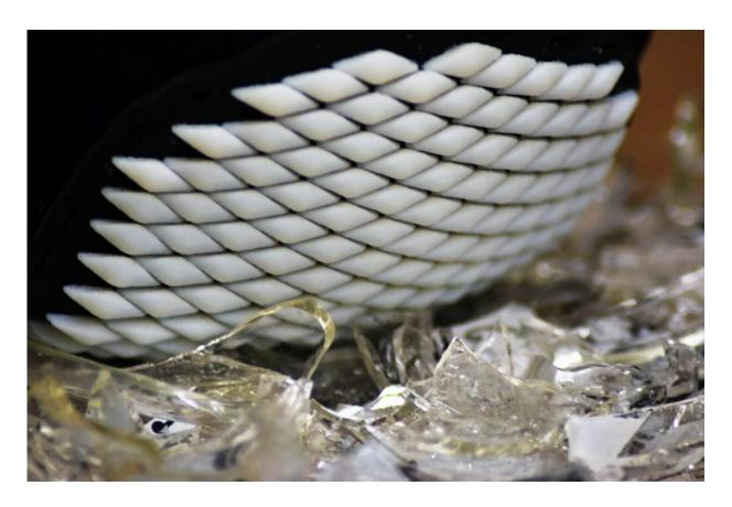
A demonstration of the 3D printed flexible armor on broken glass. Credit: Virginia Tech
