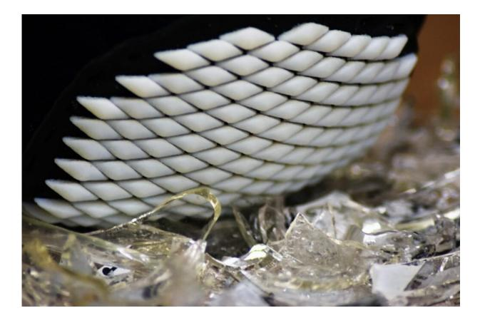
A demonstration of the 3D printed flexible armor on broken glass. Credit: Virginia Tech
