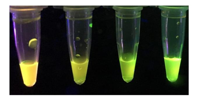
A new sensor developed by U of A chemists turns yellow or green under ultraviolet light depending on how much parathion or paraoxon is present in a sample. Credit: Chris Robidillo
