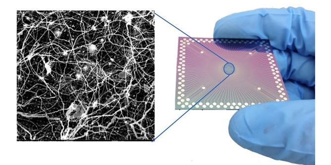
A device like the one in the study (right), and an electron microscope image showing the device's neuron-like arrangement of nanowires. Credit: Marc Roseboro/CNSI at UCLA
