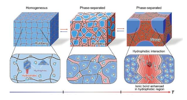
Molecular structures and the mechanisms behind instant thermal hardening of the hydrogel. Credit: Nonoyama T. et al., Advanced Materials, November 18, 2019
