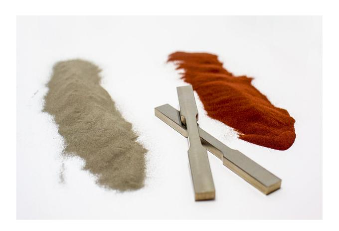
3D-printed titanium-copper bars with titanium powder and copper powder. Credit: RMIT University
