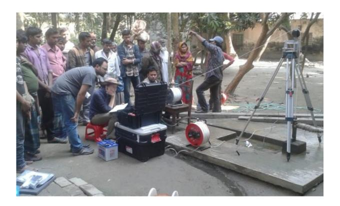
Britt Huhmann from MIT and Mahfuz Khan from the University of Delaware deploy a camera down a well to verify its depth. Credit: Lex van Geen
