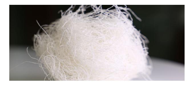
The surface of the yarn is coated with a cyclic sugar that captures the compounds into the cavities of the fibre as it swells in water. Credit: VTT
