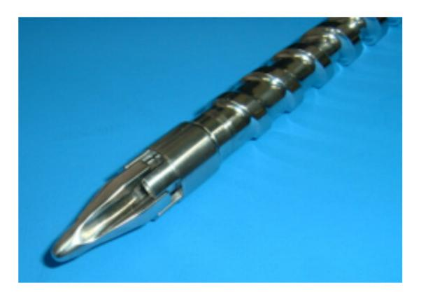
Screw for plastic injection molding, as fabricated with the developed steel. Credit: Kenta Yamanaka et al, Tohoku University
