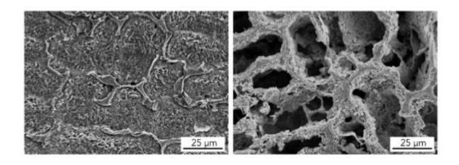
Surface appearance of the developed steel containing copper (left) and copperfree counterpart (right). Credit: Kenta Yamanaka et al, Tohoku University
