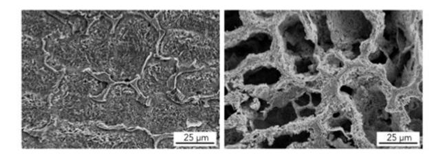
Surface appearance of the developed steel containing copper (left) and copperfree counterpart (right). Credit: Kenta Yamanaka et al, Tohoku University
